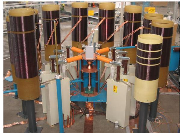
Figure 3: Standard test with  $8/20 \mu s$  pulse for V-MOV-ZnO resistor block at HVLAB.
